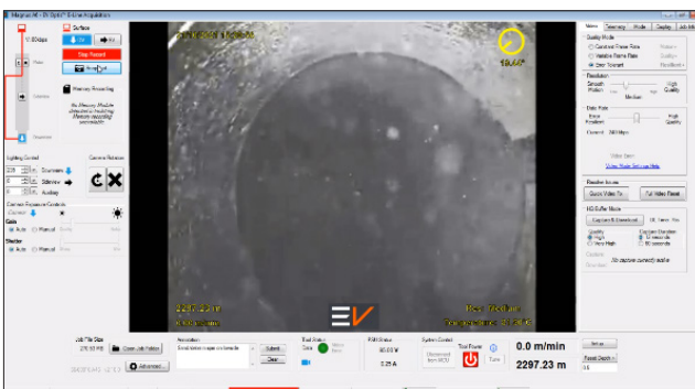
Live streamed data: LiveLink and real-time downhole camera working in conjunction to identify downhole issues
