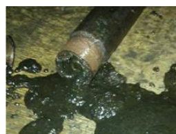
Debris recovered from well – wet scale and sand mix
