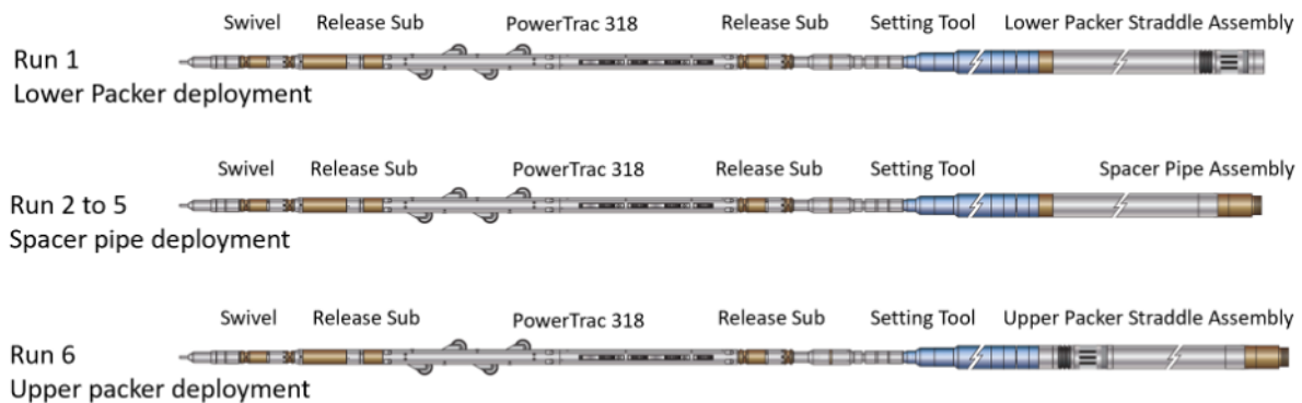
Tractor – Straddle Packer Assemblies deployment toolstrings
